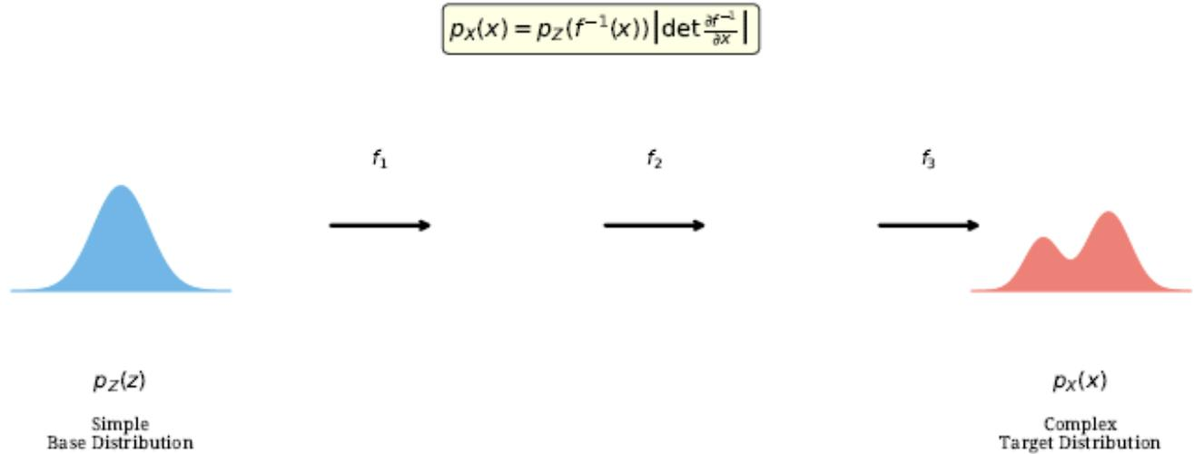
Fig. 2: Normalizing flows transform a simple base distribution (e.g., Gaussian) into a complex target distribution through a sequence of invertible transformations, enabling exact density evaluation.
