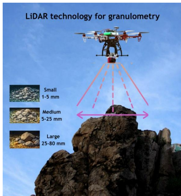
Fig. 4: Acquisition of granulometric data using drones for particle size analysis.
